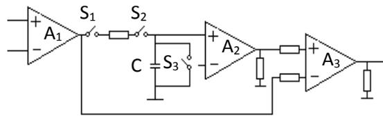
Figure 1 The diagram of automatic zero adjustment circuit
